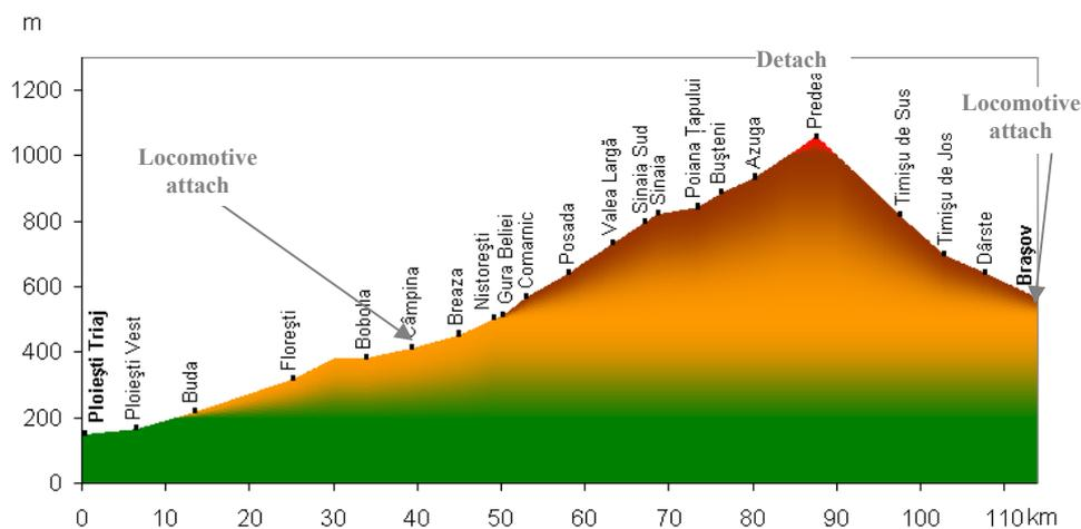
Fig. 3. Longitudinal profile of the TEN-T corridor IV and the technological operations for the pushing locomotive attaching and detaching (Source: [9])
